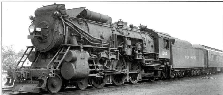
I-4-e This class consisted of locomotives with the original Type "A" superheaters and thermic syphons applied starting in 1925. New Haven #1380. NHRHTA, Inc. Collection.
