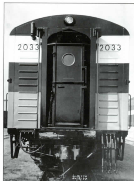
Above Left: Builder's photo of the rear of EDER-5 #2000. Above Right: Builder's photo for the rear of EDER-5a #2033. Note the detail differences between the 1957 and 1960 versions of the FL9. The lettering style is different as well. NHRHTA, Inc. Collection.
