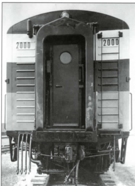
Above Left: Builder's photo of the rear of EDER-5 #2000. Above Right: Builder's photo for the rear of EDER-5a #2033. Note the detail differences between the 1957 and 1960 versions of the FL9. The lettering style is different as well. NHRHTA, Inc. Collection.
