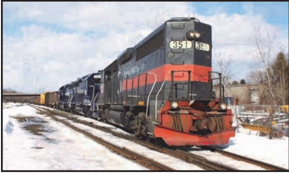
On Saturday, February 11, 2011, PanAm local PL -1 prepares to depart Plainville for East Deerfield with three engines and 45 cars. This was the first time in over fifteen years there have been three engines in Plainville at the same time. Of the three only #351 could lead because it has the necessary cab signals and ATC for operating on Amtrak. The second unit, #307, does not have these thus could only be used as a trailer, and the third unit, #352, has cab signals and ATC but was sent north dead because of outdated FRA tests. Of the 45 cars, 25 were empty LPG tank cars from Amerigas in Southington which receives a large number of these cars during the winter months. Photo: John Osmun
