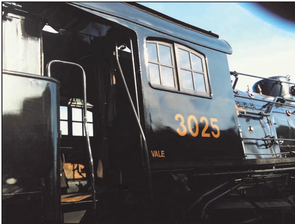
Above: Close up view of the classic New Haven style arch window cab the Valley Railroad fabricated using original New Haven Railroad drawings as a basis.
