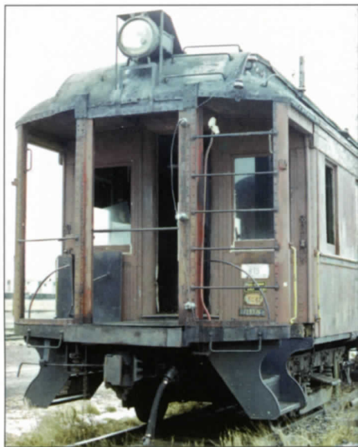
Above: W-162 in transit has the whistles removed. The base of the pipe where the left whistle was mounted is seen to the left of the headlight on the roof end cap. The right whistle was mounted on the pipe next to the right crash post (pipe extended to the bottom of the end cap). Note the supports for the headlight and cover, the ground wire and insulators running up the right crash post to the right clerestory and the grab irons on the roof cap to the right of the headlight. Below: The end windows and windshield wipers are clearly visible in this photo. Note the location of both whistles. Both photos William G. Dulmaine Collection.
