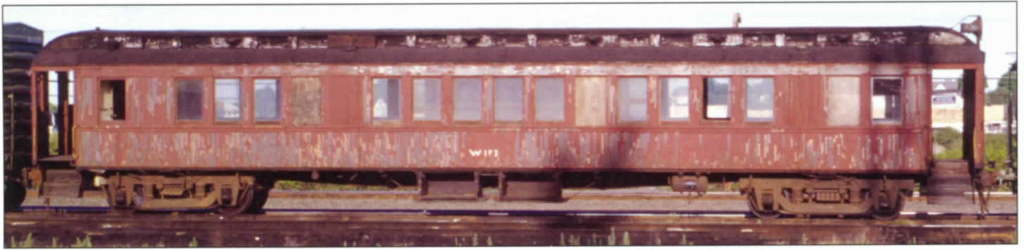
Above: this photo shows the W-162 at Northup Ave. Yards in Providence, Rhode Island in transit on PC NE-74. A former New Haven NE-6 in Penn Central livery was to the immediate right of the W-162. Note the location of the battery boxes (covers removed during transit as were the smokejacks). Also note the small air tank to the left of the "A" headlight end truck. Below: The model is shown with oversized battery boxes (supplied with the kit). Second From Bottom: Brake detail was mounted almost directly across from the battery boxes and centered on the cars number. Bottom: This photo shows the small air tank installed on the finished model.
