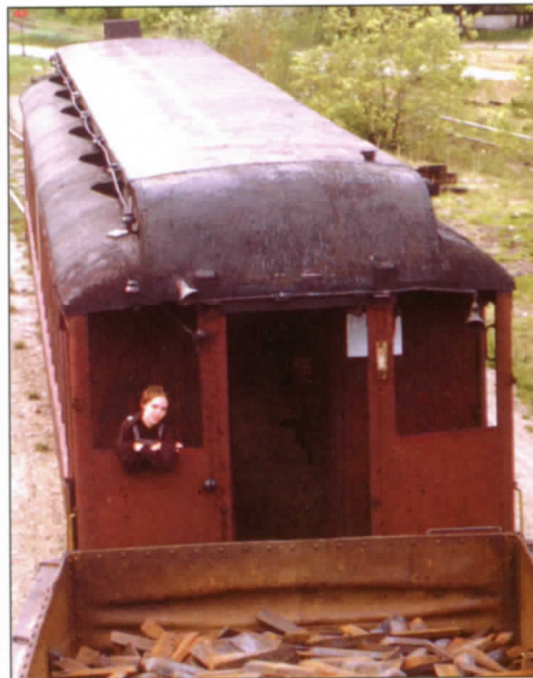
Below Left: Photo of ground wire running from smokejack to the frame. Below Right: The ground wire with insulators is shown running the length of the clerestory and down the end of the car. Also note the water filler cap over the lavatory and the floodlights above the openings on the car end. Above Right: Note Globe vent, filler cap (on roof) and an electric plug cap is below the window.
