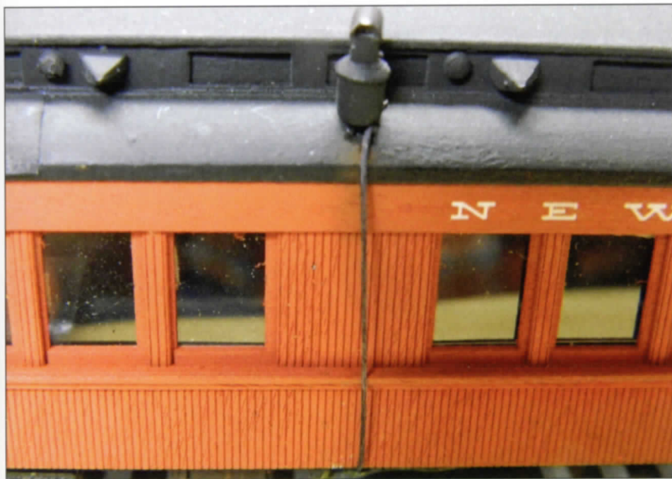
Below Left: Photo of ground wire running from smokejack to the frame. Below Right: The ground wire with insulators is shown running the length of the clerestory and down the end of the car. Also note the water filler cap over the lavatory and the floodlights above the openings on the car end. Above Right: Note Globe vent, filler cap (on roof) and an electric plug cap is below the window.
