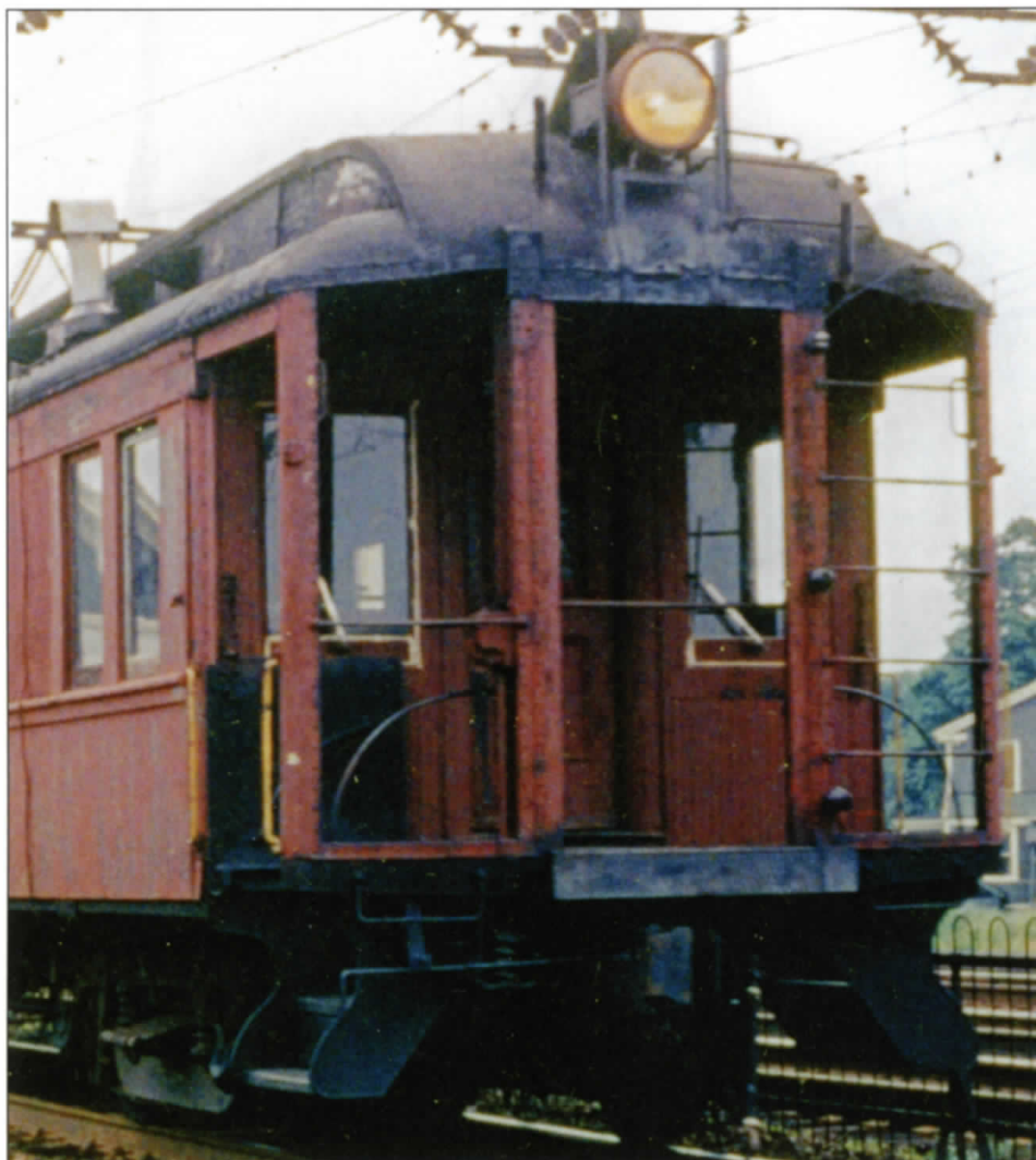
Above: W-162 in transit has the whistles removed. The base of the pipe where the left whistle was mounted is seen to the left of the headlight on the roof end cap. The right whistle was mounted on the pipe next to the right crash post (pipe extended to the bottom of the end cap). Note the supports for the headlight and cover, the ground wire and insulators running up the right crash post to the right clerestory and the grab irons on the roof cap to the right of the headlight. Below: The end windows and windshield wipers are clearly visible in this photo. Note the location of both whistles. Both photos William G. Dulmaine Collection.
