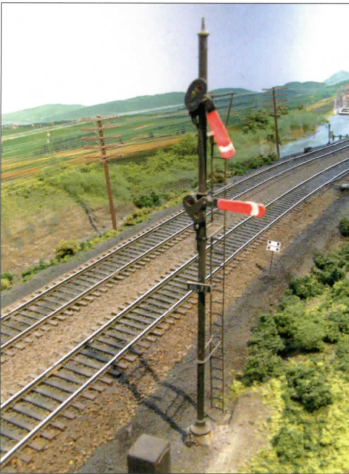
Above: INTERLOCKING DRAWBRIDGE SIGNAL Rounded blade ends and boards vertical above each other show a restrictive signal. Aspect in photo is clear. Above Right: DISTANT OR APPROACH SIGNAL approach is indicated by lower board using yellow fish tail. Below Right: BLOCK SIGNAL red board with pointed end. Note: by 1947 some block signals were lower quadrant while others were upper quadrant.
