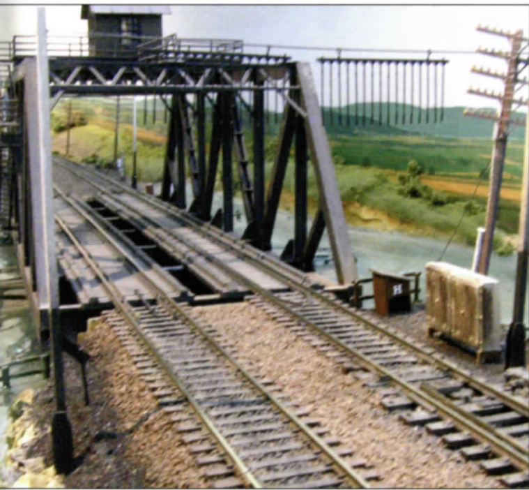
Left: SWING BRIDGE AND APPROACH DETAILS Telltales and support poles at the approach to the swing bridge at Mystic, Connecticut on my layout. Above: FIRE HOSE BOX used in such areas as draw/swing bridges, towers, etc. Below Left and Below Right: RELAY CASE (on opposite approach to the bridge) for signals and derail, also showing circuit breaker box (small vertical box on the utility pole).
