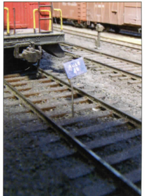
Above: RAILROAD CROSSING DETAILS whistle post for grade crossing not visible beyond the curve and cross bucks guarding the crossing in the foreground. Note the planked crossing on the rural dirt road. Left: This view is from the other side of the crossing above. FLANGER SIGN for grade crossing in the distance. Below: RULE 26 BLUE FLAG POST was blue metal flag and post. In 1947 "RULE 26" was painted on the flag.
