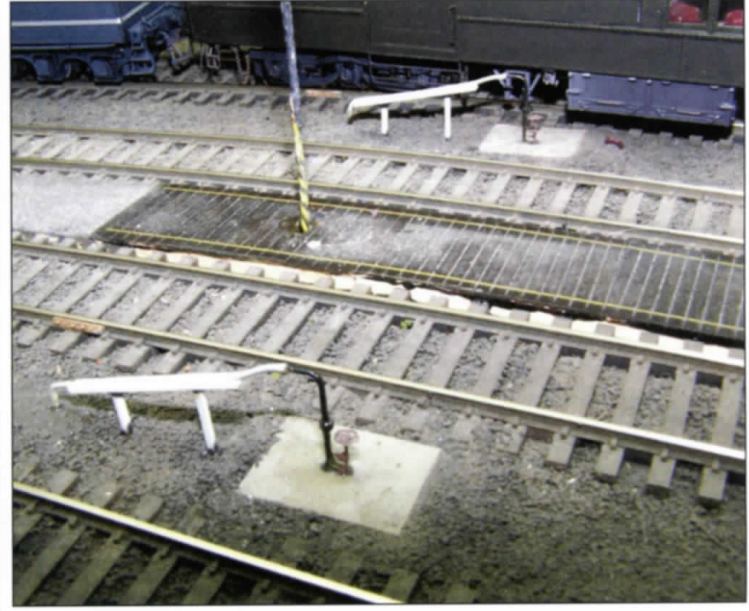
Above Left: ORMS STREET TOWER AND TELLTALES at Smith St. overpass in Providence, Rhode Island. Above Right: CAR WATERING STATIONS at Providence, Rhode Island station. Hoses are supported in white troughs.
