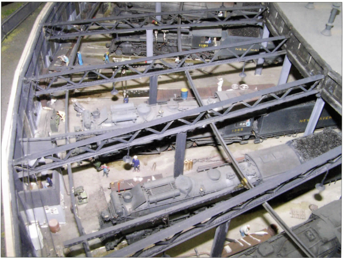
Above: General interior view of the Charles St. engine house. The foreman's office is in the lower left of the photo. The locomotives from top to bottom L-1 2-10-2 #3201, H-1 4-4-2 #1101, I-4 4-6-2 #1388 and I-4 4-6-2 #1391. Below: Charles St. engine terminal showing water stand pipe. Bottom Left: Interior of Charles St. engine house with foreman's office and small lathe at lower left. Locomotives visible from top to bottom I-4-c 4-6-2 #1357, R-2a 4-8-2 #3505 and R-3a 4-8-2 #3553.
