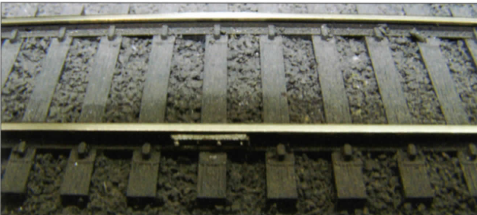
Below: FOUR BOLT FISH PLATE used on secondary main tracks, yard tracks and sidings.
