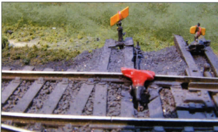
Above: DWARF SWITCH STAND on yard tracks. Targets usually red and lunar white or yellow and purple (era 1948). Below: SIDING DERAIL AND THROW STAND New Haven derrails were red.
