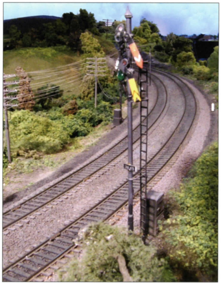
Above: INTERLOCKING DRAWBRIDGE SIGNAL Rounded blade ends and boards vertical above each other show a restrictive signal. Aspect in photo is clear. Above Right: DISTANT OR APPROACH SIGNAL approach is indicated by lower board using yellow fish tail. Below Right: BLOCK SIGNAL red board with pointed end. Note: by 1947 some block signals were lower quadrant while others were upper quadrant.
