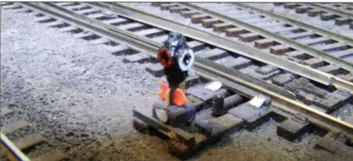
Above: DWARF SWITCH STAND on yard tracks. Targets usually red and lunar white or yellow and purple (era 1948). Below: SIDING DERAIL AND THROW STAND New Haven derrails were red.
