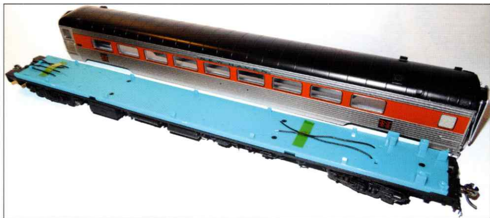
The unnamed version right out of the box shows off the one-piece body construction of the parlor and the pre-drilled floor for doing the 26C-14L or 36C versions.
