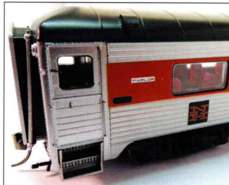
The steps were replaced and the stirrups removed as unnecessary when the skirts were eliminated. Photo: Paul Cutler III
