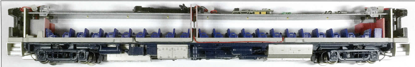
Above: This photo shows the interior arrangement of electronics and seating in the new Budd car by Rapido. Below: The floor is raised slightly to accommodate the drive shafts to the trucks. This is not visible from the outside of the car.
