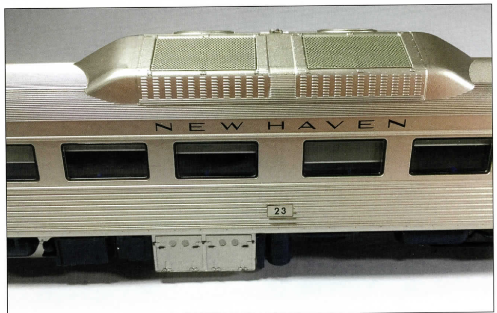
Below: The rectangular opening centered on the top of the blister is indeed correct. This recess was indeed left open on most RDCs produced. Some railroads may have covered this area with a grate, as most model manufacturers have in the past.
